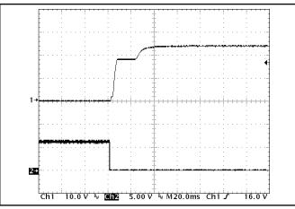
**Figure 10:** Turn-on transient at zero load current (20 ms/div). Ch 1: Vout (10V/div) Ch 2: ON/OFF input (5V/div)
