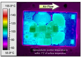
Figure 6: Thermal plot of converter at 5 amp load current (120W) with 55°C air flowing at the rate of 200 LFM. Air is flowing across the converter from input to output (nominal input voltage).
