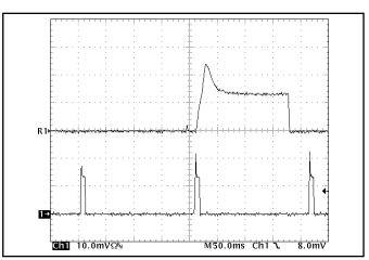
**Figure 18:** Load current (5A/div) as a function of time when the converter attempts to turn on into a 1 m $\Omega$  short circuit. Top trace (2.5ms/div) is an expansion of the on-time portion of the bottom trace.
