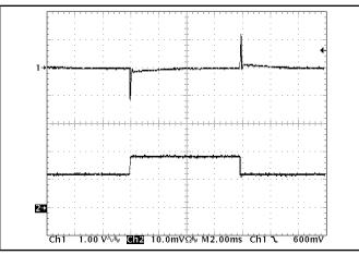
**Figure 11:** Output voltage response to step-change in load current (50%-75%-50% of Iout(max);  $dI/dt = 0.1A/\mu s$ ). Load cap:  $10\mu F$ , 100 m $\Omega$  ESR tantalum capacitor and  $1\mu F$  ceramic capacitor. Ch 1: Vout (1V/div), Ch 2: Iout (2A/div).
