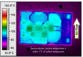
*Figure 8:* Thermal plot of converter at 5 amp load current (120W) with 55°C air flowing at the rate of 200 LFM. Air is flowing from pin 3 to pin 1 (nominal input voltage).
