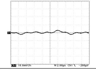
**Figure 15:** Input reflected ripple current,  $i_s$ , through a 10  $\mu$ H source inductor at nominal input voltage and rated load current (20 mA/div). See Figure 13.
