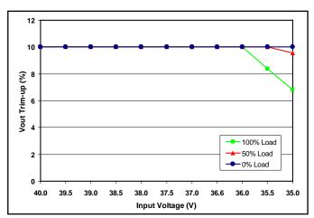
*Figure 12:* Percentage of output voltage trim-up that can be achieved at various input voltages from Vin 35V-40V and output loads of 0%, 50% and full load.
