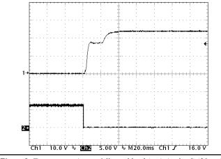
*Figure 9:* Turn-on transient at full rated load (resistive load) (20 ms/ div) Input voltage pre-applied. Ch 1: Vout (10V/div). Ch 2: ON/OFF input (5V/div)
